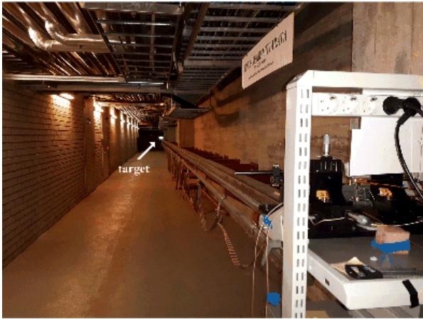
Fig. 9. Pulsed TOF laser radar measurement track.
