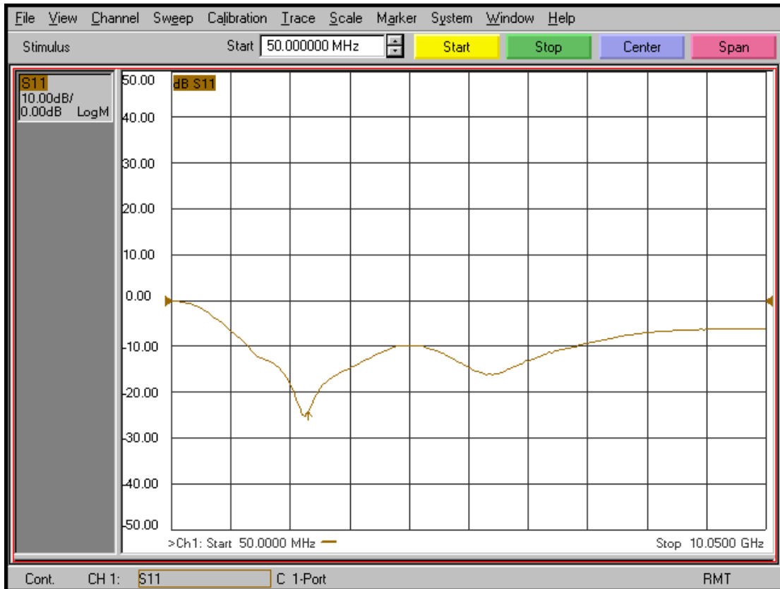
Fig.5.2.5 The measured S11 of LNA at the input of the receiver
