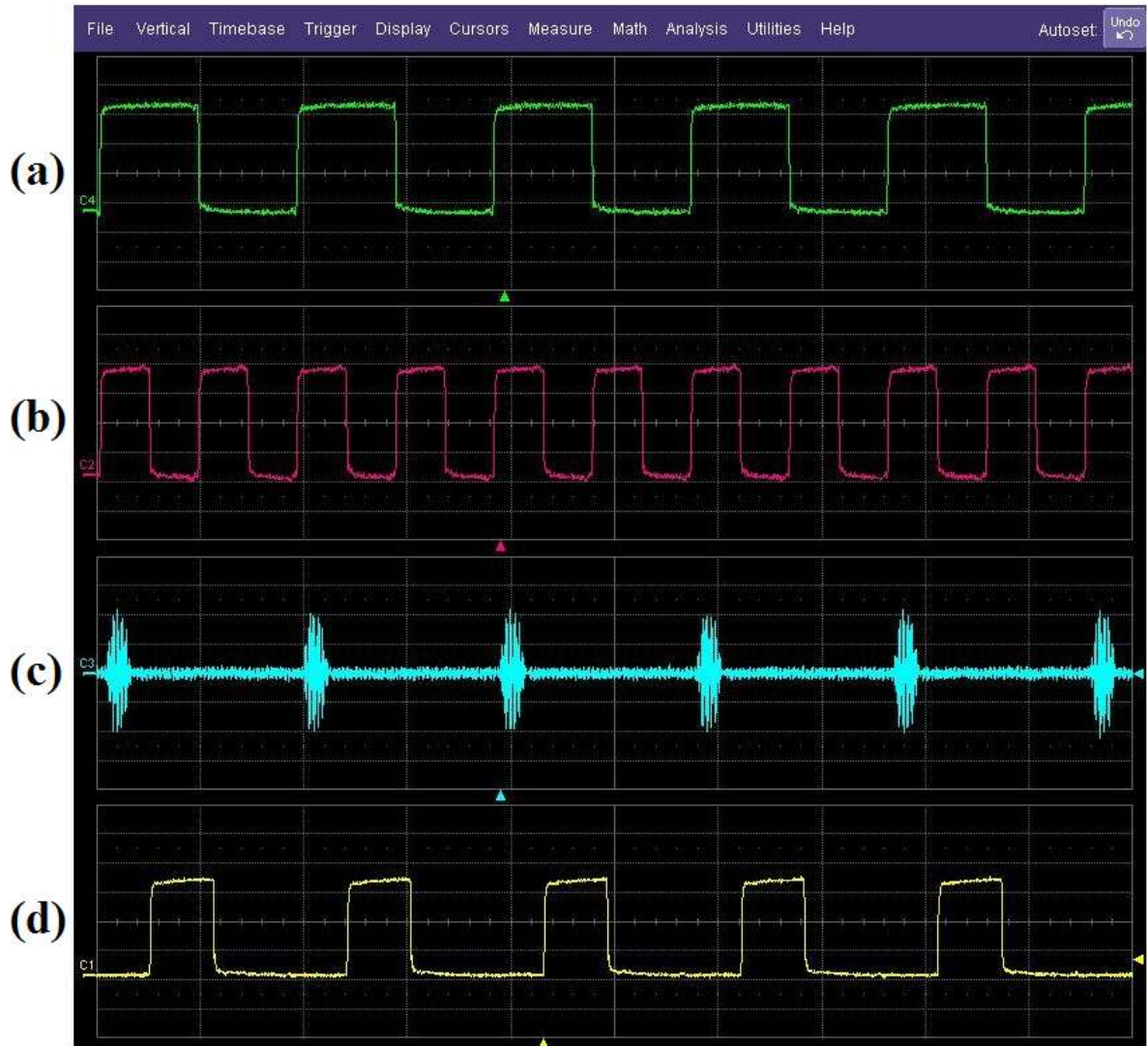
Fig.5.2.6 (a) The data input of the transmitter; (b) The clock input of the transmitter; (c) The received pulse train of the receiver; (d) The output of the receiver. (measurement)
