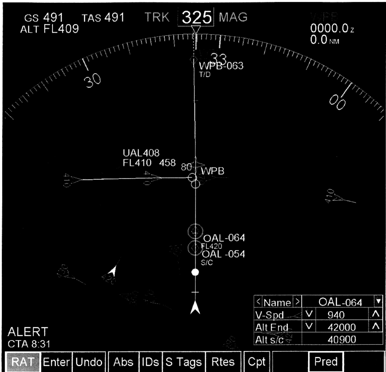
Figure 8. To prevent confusion between Primary alerts and ARAT alerts, primary alerts always had yellow tags up and the point of loss of separation was presented until the alert was solved. ARAT alerts were only identified by the alert symbols (e.g., filled chevron to left of ownship). ownship's symbol would only return to white if the proposed path was clear of the primary alert and all other aircraft.
