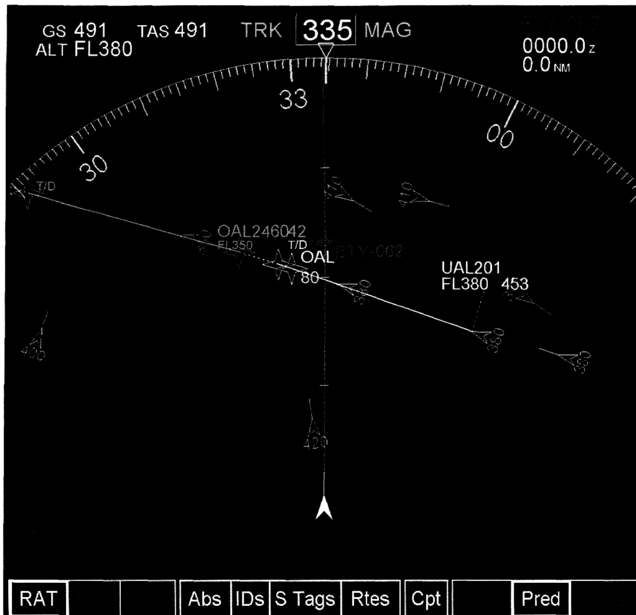
Figure 4. Three dimensional flight plan information was available on all aircraft within the supersector. A flight plan is presented for UAL201. This aircraft is currently co-altitude with ownship and is color coded white. The flight plan shows that it will start descending after crossing OAL and it will level off below ownships current altitude. Therefore, the portion of the flight plan behind OAL is white (co-altitude) and the portion after OAL246042 is green (below ownship altitude). The dashed portion between the top of descent (T/D) and OAL246042 represent the altitude change segment and the destination flight level of the aircraft is presented at the latter waypoint (FL 350).
