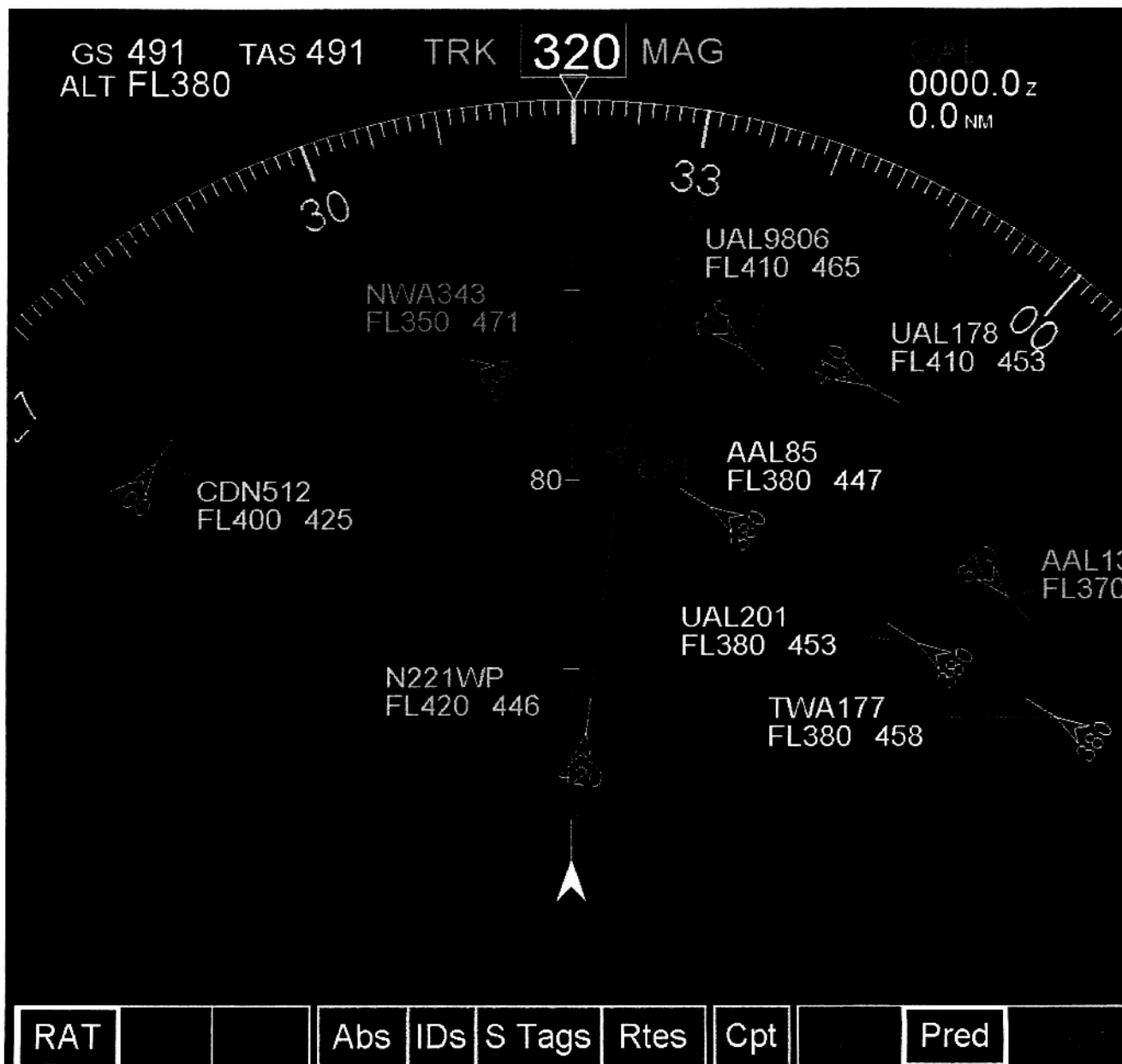
Figure 6. All Ids on was an option available to the crews. By clicking on the Ids button on the on screen toolbar or by pressing the ID button on the control panel, all Ids can be turned on/off, with the exception of any aircraft that is currently at any SA level (e.g., UAL201 is currently in an SA1 and is presented in yellow).
