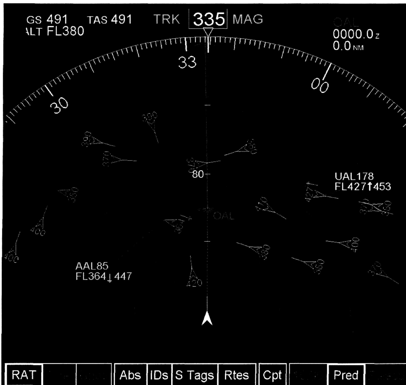
Figure 3. Color was used to display basic categorical information for relative altitude.* Aircraft above ownship current flight level (38,500) are color coded blue. Aircraft below ownships current flight level (37,500) are color coded green. The aircraft with tags are climbing and descending, as indicated by the arrow on the tail tag of the aircraft. Also, as shown, the arrow is placed next to the current flight level in the extended tag.
