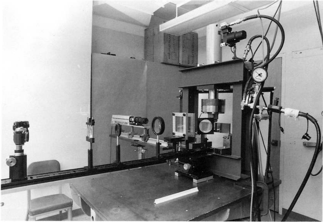
Fig. 6. Experimental arrangement for fracture experiment using CGS.
