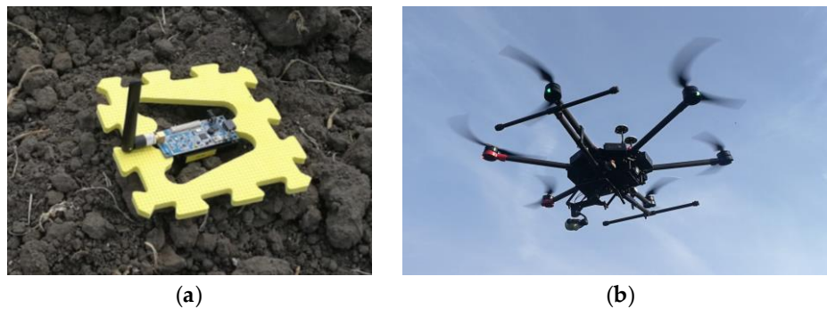
Figure 12. Equipment used in the experimental run. (a) Ground sensor node; (b) UAV.
