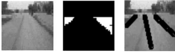
Figure 29. Segmentation and edges estimation on cloudy conditions.
