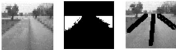
Figure 30. Segmentation and edges estimation on rainy conditions.
