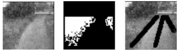
Figure 28. Segmentation and road edges estimation on a rural path without asphalt.
