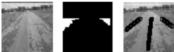
Figure 31. Segmentation and road edges estimation on post-rainy conditions.
