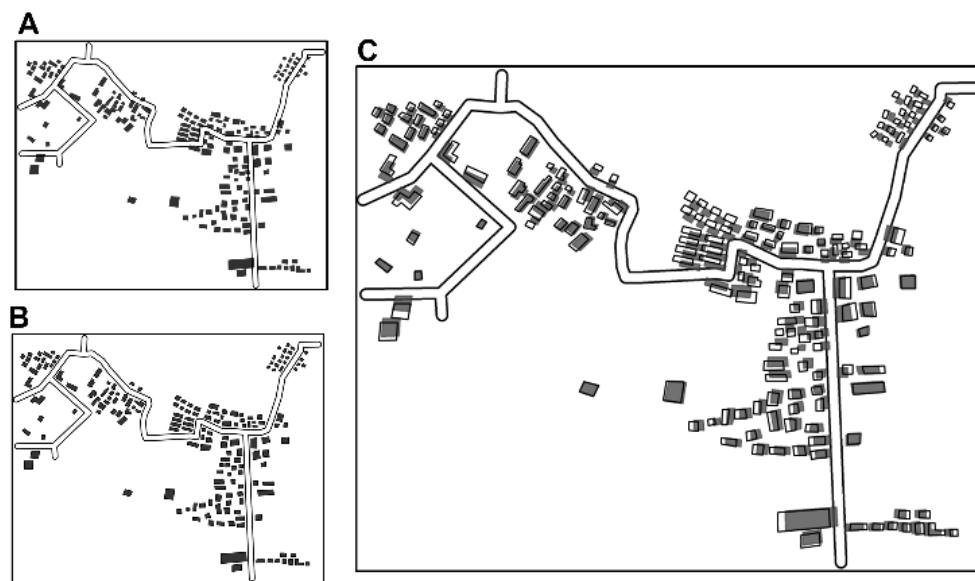
Figure 10. Visual result of data set B. (A) Initial situation (1:25 000), (B) resultant situation (1:25 000), and (C) comparing the initial and final states (1:25 000 enlarged to 1:12 500).
