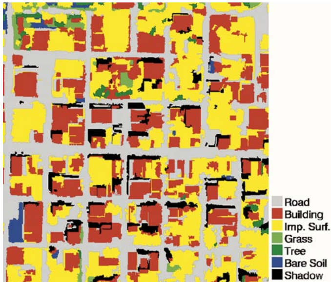
Fig. 6. Object-based classification of dense urban area shown in Fig. 1 using segmentation image shown in Fig. 4 and fuzzy-logic pixel-based classification shown in Fig. 3.
