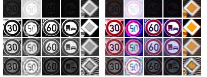
Fig. 2. Five gray-scale (left) and color (right) traffic signs normalized differently. Original images (first row), \pm 1\sigma normalization (second row), \pm 2\sigma normalization (third row) and CLAHE (fourth row).
