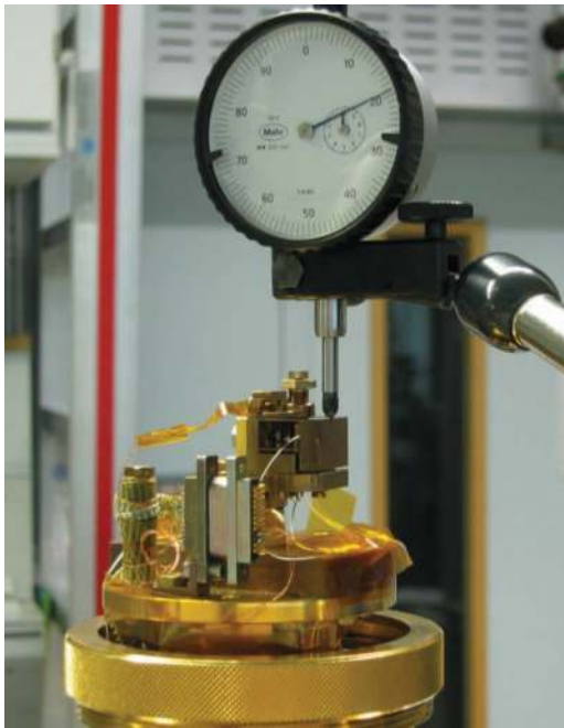
FIG. 2. Test setup for our dilatometer with a standard dial gauge. The sensors tip of the dial gauge is set perpendicular to the upper surface of the movable part.
