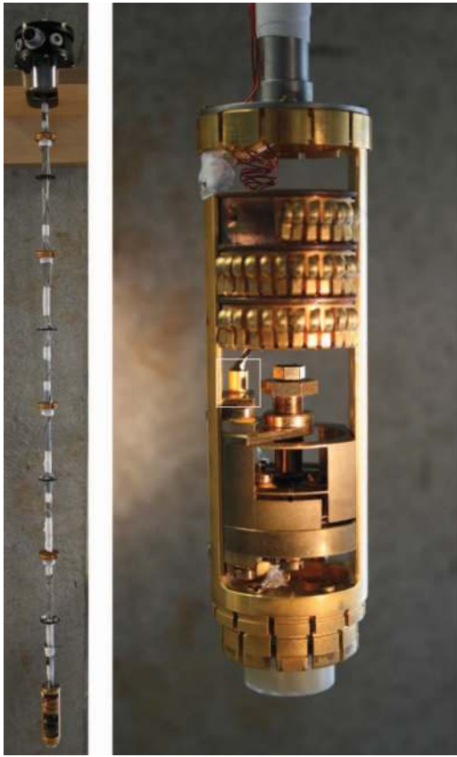
FIG. 6. Left: The complete measuring probe with gold plated thermal anchors and connectors for capacitance and temperature measurements. Right: Dilatometer within the multi-functional chamber. The position of the thermometer is highlighted by the white frame.
