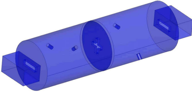
Fig. 2. Dual-mode circular-waveguide filter geometry. Cavity length: 43.87 mm. Radius: 14 mm. Iris thicknesses: 1.5 mm. Slot lengths: 10.05 mm. Slot widths: 3 mm. Arm widths: 2 mm. Horizontal arm length: 7.65 mm. Vertical arm length: 8.75 mm. Tuning screw depth: 3.59 mm. Coupling screw depth: 3.31 mm.
