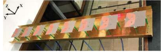
Fig. 7. Prototype of the antenna array with 1 \times 8 elements.
