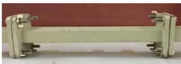
Figure 21. TRL calibration of waveguide.
