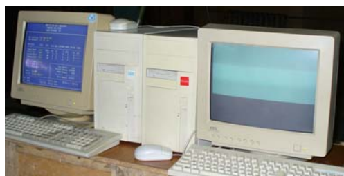
Fig.11. Different damage effects are detected for desktop computers: stopping (left computer, the clock in BIOS stops, operation restores after reload), graphics card malfunction (right computer, operation restores in several hours).
