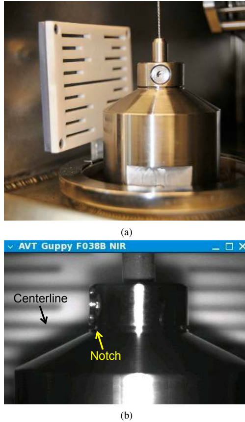
Figure 7: Two images of the weight in its “tare” position, in which the notch in the weight’s neck is aligned with the long centerline in the camera backdrop. Photo (a) shows the weight and rulered backdrop inside the MiniCal housing, while screenshot (b) shows the same scene as viewed through the camera. The backdrop’s hash marks are spaced at 5 mm intervals.
