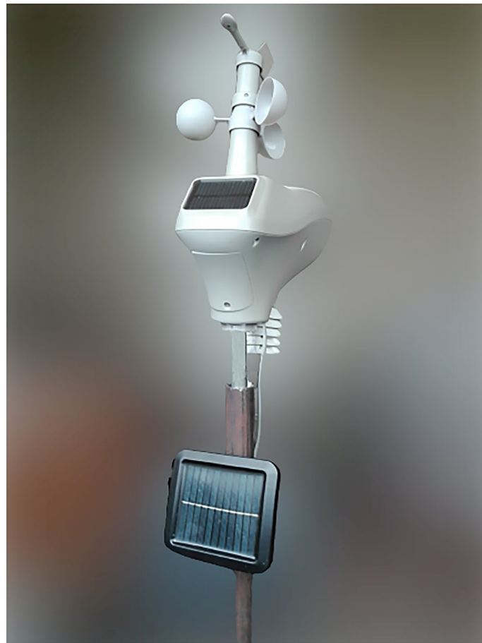
Figure 4. PV panel and weather station.
