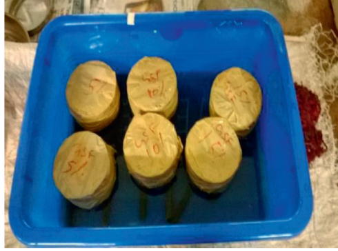
FIGURE 6: Specimens for the sorptivity test.
