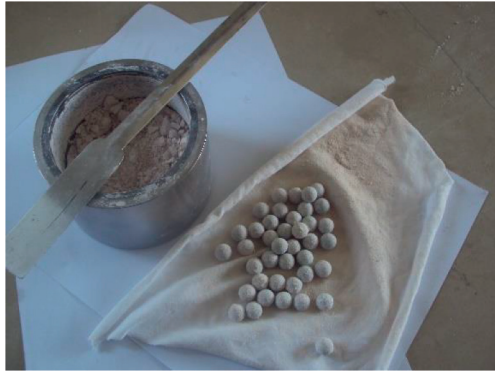
FIGURE 1: Zirconium balls and metakaolin during grinding.
