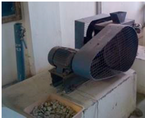
FIGURE 3: Jaw crusher for crushing tiles.
