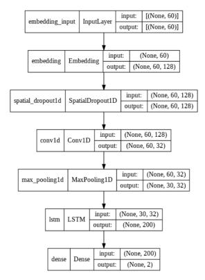
Figure 3. CLSTM model architecture.
