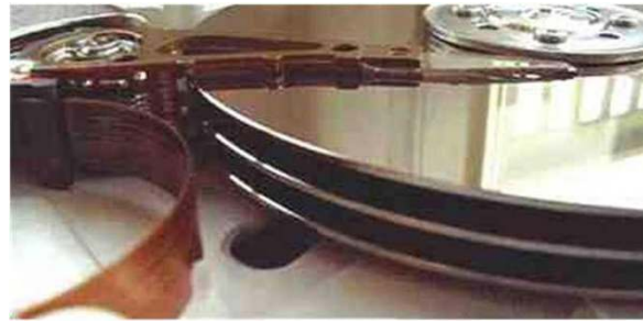
Figure 1 Computer Hard Drive. Computer Hard drive showing multiple disks and read/write head. Picture from "How things Work" by Marshall Brain.
