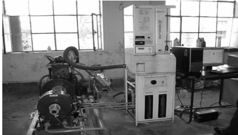
Plate 1. Variable compression ratio compression ignition engine experimental setup
