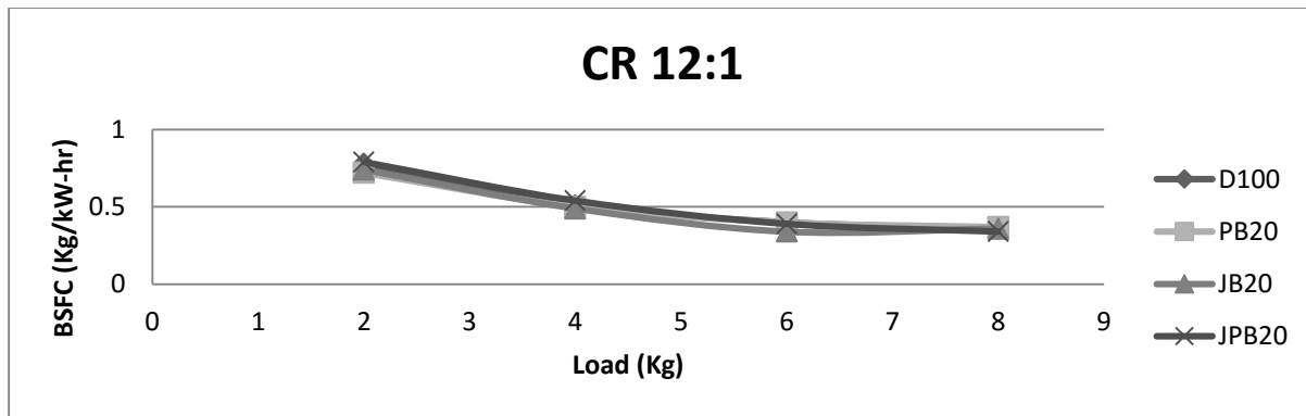
Figure 7. Variation of Brake specific fuel consumption with respect to load for 12cr
