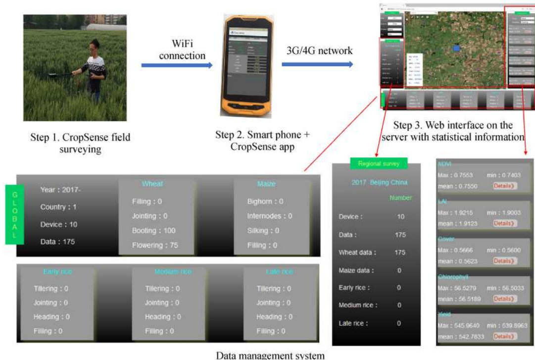
Fig. 6 Workflow of the CropSense system developed by NERCITA, China
