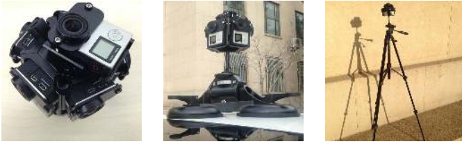
Fig. 1. Capture device. Left: camera rig holding multiple cameras. Center: rig mounted on a car. Right: rig mounted on a tripod.
