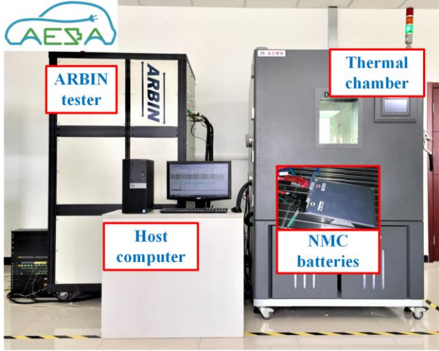
Figure 1 Battery test platform.
