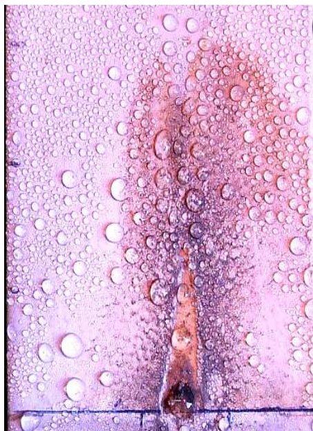
Fig. 58: Appearance of test sample AC4-A6 (not abraded) after washing.
