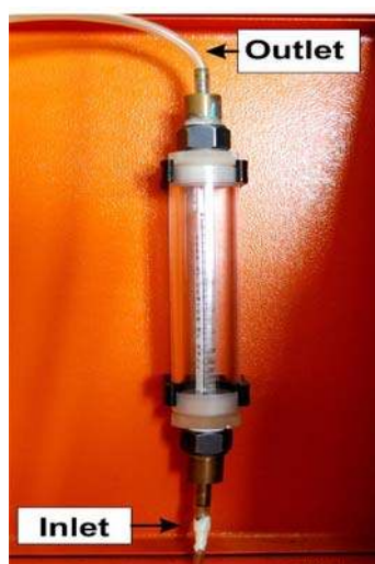
Fig. 32: Flow meter as installed in apparatus.
