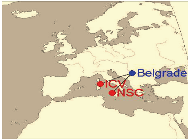
Fig. 1. Great Circle Paths (GCP) of subionospheric propagating VLF signals recorded at the Belgrade station. The receiver is continuously monitoring the amplitude and phase of coherent and subionospheric propagating VLF signals operated in Sicily at 45.90, kHz and Isola di Tavolara at 20.27 kHz.
