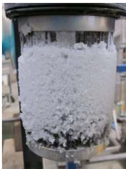
Fig. 1 Clogging of a typical fuel filter [32]
