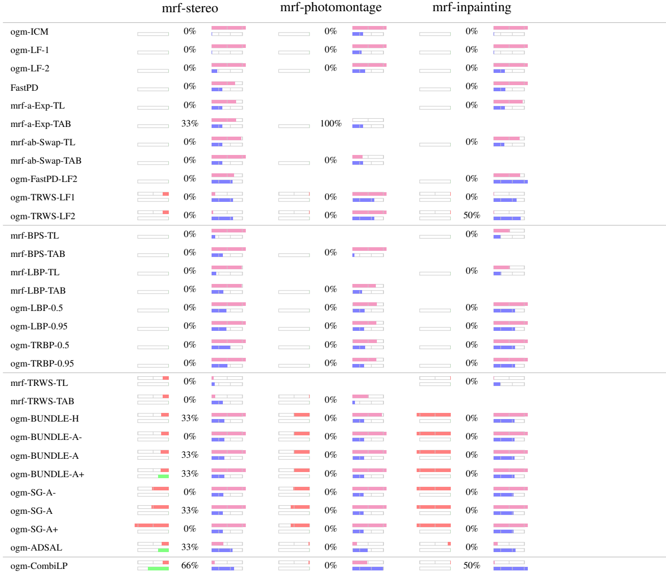
Figure 14: Results for grid structured models with four-pixel neighborhood-system and truncated convex regularization from [66]. See Fig. 13 for the legend. For all models local polytope relaxations give good lower bounds. However, extracting a integer solution from the fractional one can be very difficult, especially for the photomontage instances, where soft constraints renders linear programming relaxation harder. FastPD and \alpha -expansion are the first choice if fast optimization is required. For stereo- and inpainting problems LP-relaxations as obtained by TRWS have given best results – especially when followed by lazy flipping post processing. For some instances we were able to solve them to optimality by CombiLP but often need more than 1 hour.
