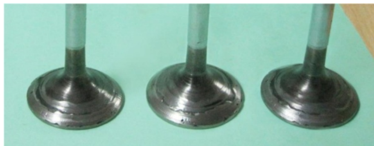
Fig. 2 A photographic view of the few workpieces after rough grinding
