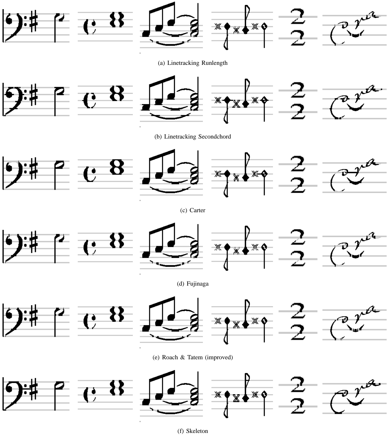
Fig. 11. Details of the results of different staff removal algorithms on our undeformed test set. Removed pixels are marked grey. The details show (from left to right): bass clef followed by sharp and half note, cut time symbol followed by a chord of two whole notes, beamed eighth notes tied to a chord of half notes, 16th-century music typeface, modern guitar tablature, 17th-century French lute tablature.
