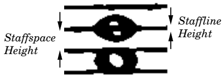
Fig. 1. The characteristic page dimensions staffline_height and staffspace_height .
