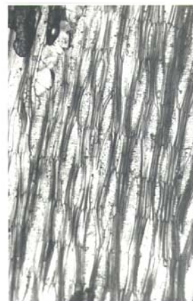
(b) Tangential Longitudinal Section of Triplochiton scleroxylon (Softwood) with multi-seriate rays. (x144)
