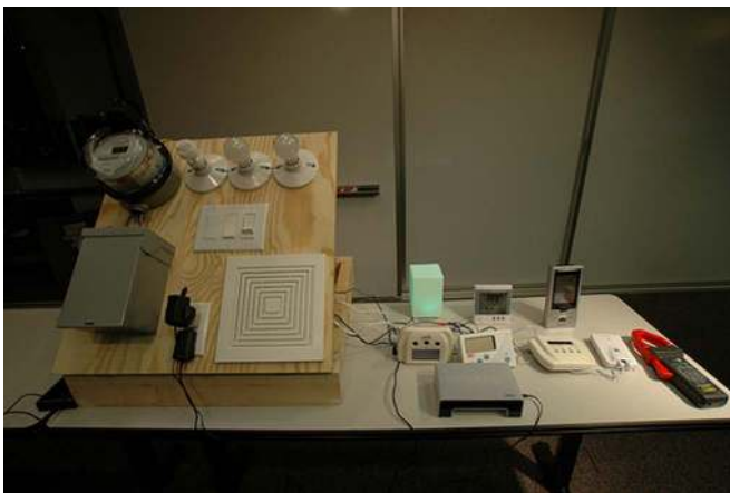
Fig. 2. Device testing using a simulated residential display board.
