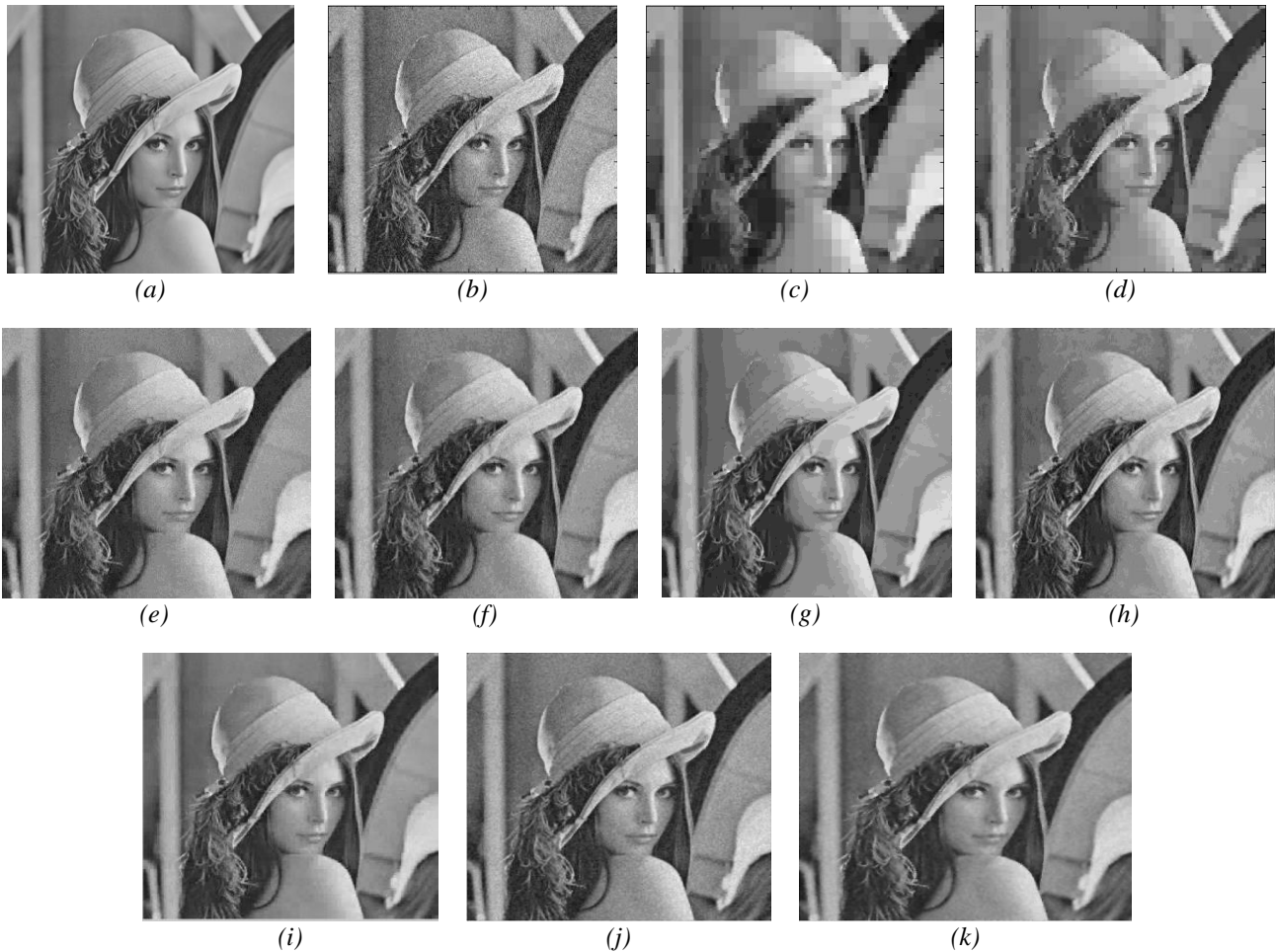
Fig.10. Denoising of test image Lena: (a) Original Image; (b) Image corrupted with Gaussian noise with std. deviation = 20; (c) Visu Shrink using hard thresholding; (d) Visu Shrink using soft thresholding; (e) Sure Shrink using soft thresholding; (f) Bayes Shrink using soft thresholding; (g) Prob Shrink; (h) Block Shrink; (i) Neigh Shrink Sure; (j) Median filter; (k) Wiener filter
