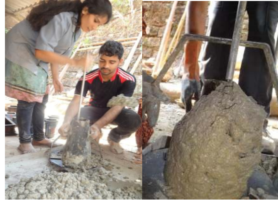
Fig 2: Slump test carried out on concrete
