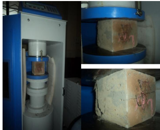
Fig 3: Compressive Strength Test on Cubes
