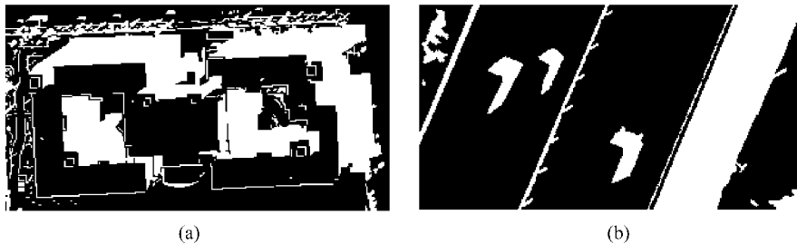
Fig. 4. Manually interpreted shadow masks (white area) as ground truth of shadow regions. (a) Shadow of the image in Fig. 3(a). (b) Shadow of the image in Fig. 3(b).
