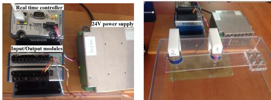
Fig. 2 Active vibration attenuation in a smart beam.
