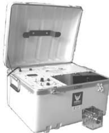
Figure 1 Liquid Dielectric Test Set, Model LD60 for breakdown measurement.
