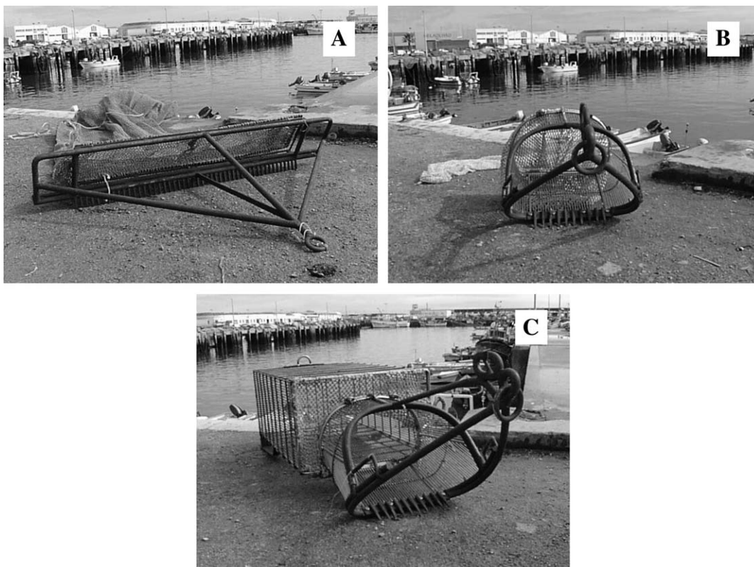
Figure 1. Photographs of the three dredge types used in the S. solida Portuguese fishery. (A) North dredge (ND); (B) traditional dredge (TD); (C) grid dredge (GD).
