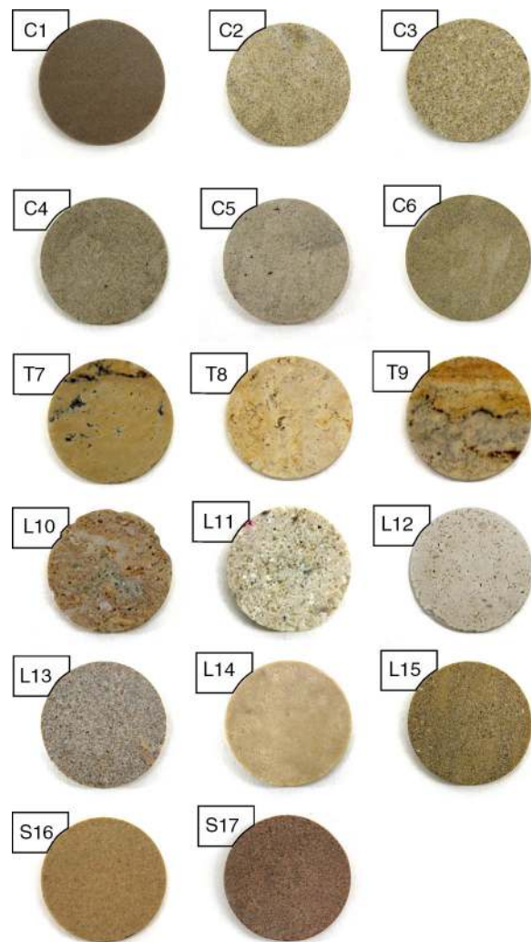
FIGURE 1. Image of the studied samples. C: biocalcarenes. T: travertines. L: allochem limestones. S: silica cement sandstones.
