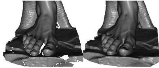
Fig. 5. Hole-filling method which applies volumetric diffusion. The method presented by Davis et al. (2001).
