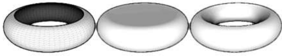
Fig. 6. Hole-filling of a torus using 3D space decomposition in atomic volumes. The image on the far left shows the original torus that must be repaired. The other two images are two different solutions produced by the algorithm. The method presented by Podolak and Rusinkiewicz (2005).
