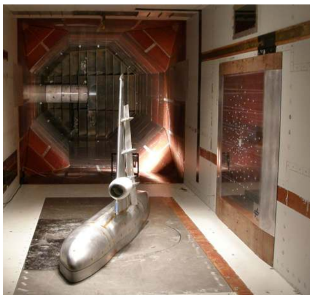
Figure 1. Photo of the test section with the array mounted on the side wall and the DO-728 semispan model in the center, view in the flow direction.
