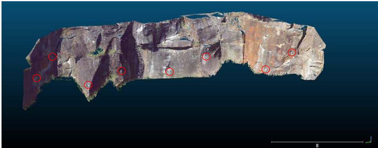
Figure 2. Reference model obtained with the TLS and locations of the eight GCPs (red circles)
