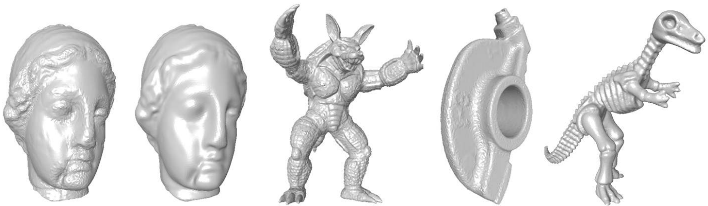
Fig. 4. Samples of the general-purpose corpus. From left to right : Venus with noise on rough areas, Venus with global smoothing, Armadillo with noise on smooth areas, RockerArm with noise on intermediate areas, Dyno with smoothing on rough areas.
