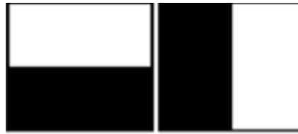
Figure3 Haar wavelet types used for SURF
