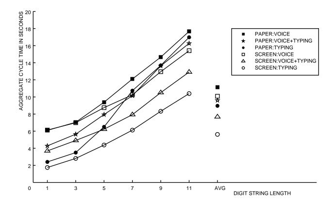
The aggregate cycle time is shown for each input condition (voice, voice with typing and typing) for both experiments. The plot includes each digit string length plotted separately; AVG denotes the overall average for a condition.
