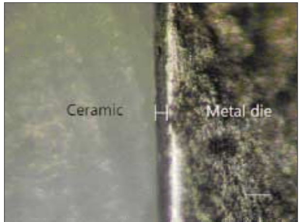
Fig. 4. Marginal discrepancy evaluation using a measuring microscope. (original magnification × 100, white bar represents 100 μm)
