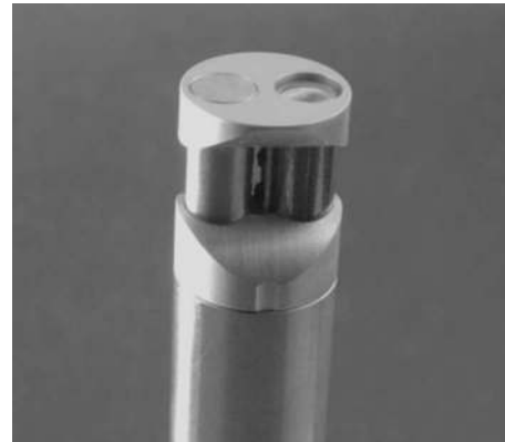
FIG. 2. A Microflow 1/2 in. sound intensity probe. The particle velocity sensor can be seen on the solid cylinder to the right; the electret microphone is mounted inside the other cylinder.
