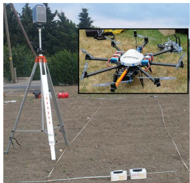
Figure 4: The TLS and UAV instruments used in this experiment.
