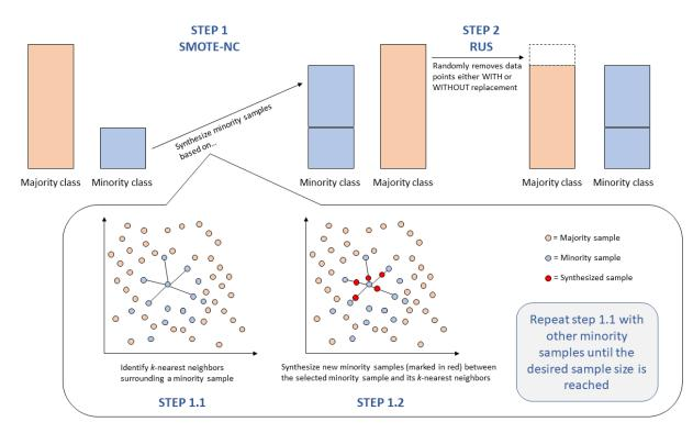
Figure 3. Hybrid resampling process.
