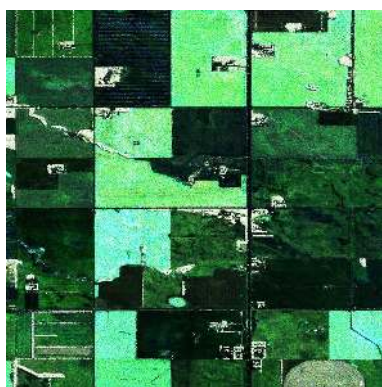
Figure 3. color composite of coherency matrix (RGB: T 11 , T 22 , T 33 ), acquired on 2012/07/17
