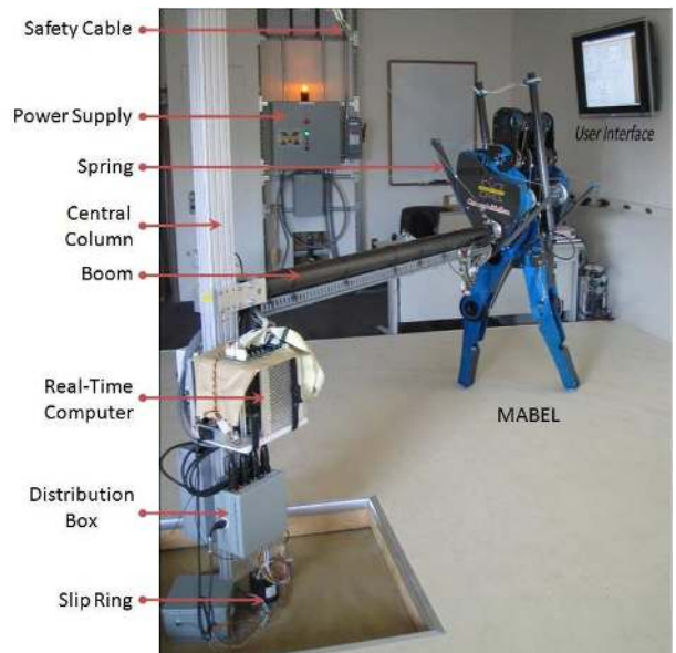
Fig. 10. Experimental setup of the bipedal testbed MABEL.
